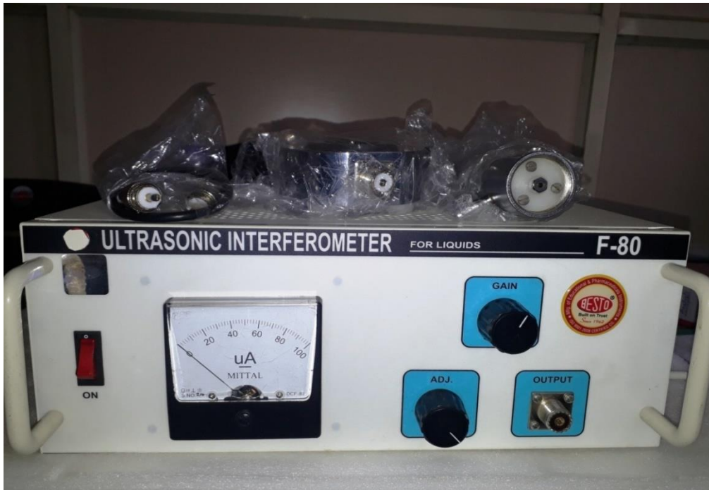
Ultrasonic Interferometer Frequency 2MHz
